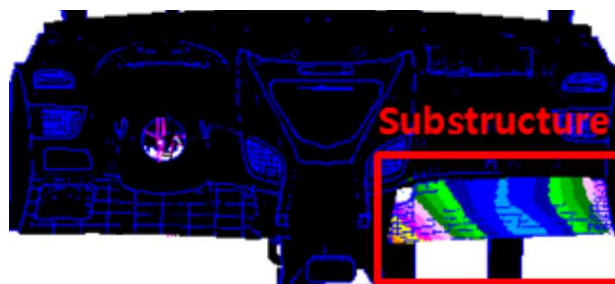
Fig. 5 Sub-structure analysis result
