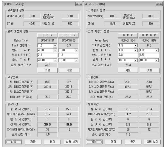
Fig. 12. The evaluation of protection coordination between recloser and customer relay ; without DG(A), with DG(B)
