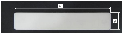
Fig. 6 Position for shrinkage measurement
