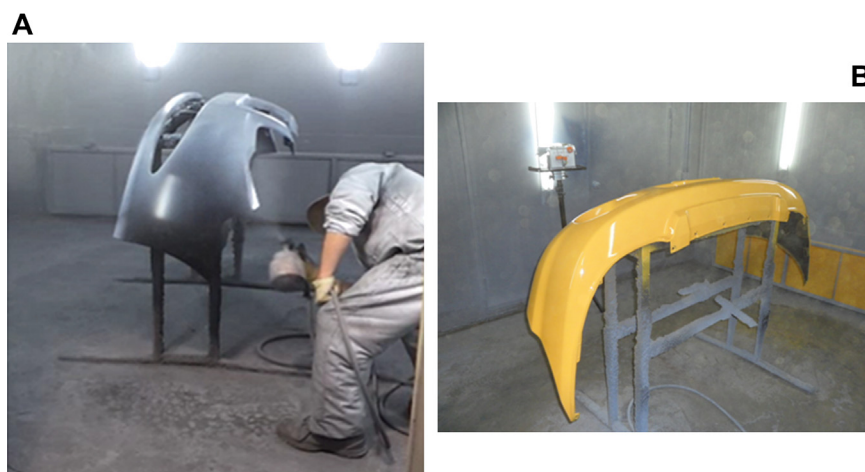
Fig. 1. The spray painting process. (A) Gray paint. (B) Yellow paint.
