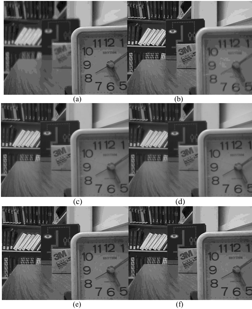
Fig. 4. The fusion results of different lowpass coefficient fusion algorithms: (a) Focus on the right; (b) focus on the left; and (c)–(f) fused images using the average scheme, directional vector maximum choosing scheme, local gradient energy maximum choosing scheme, and the proposed lowpass subband fusion rule.
