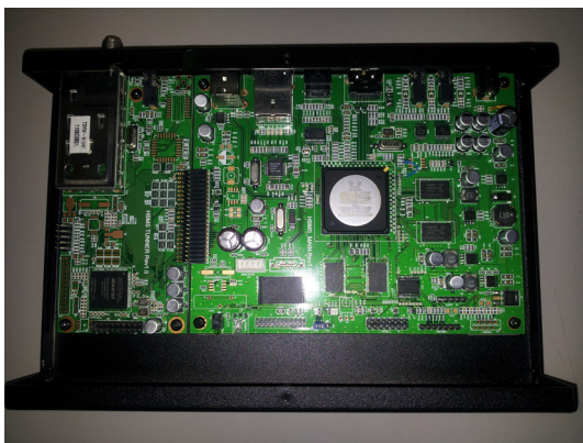
[Fig. 3] Developed board for the receiving controller
