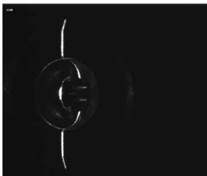
Fig. 16 Images of lasers projected on punch head
