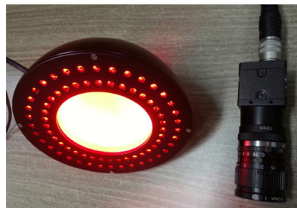
Fig. 1 CCD camera and dome light
