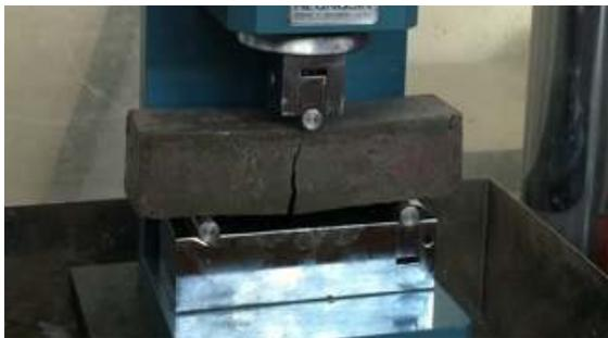
(b) Flexural failure of mortar
