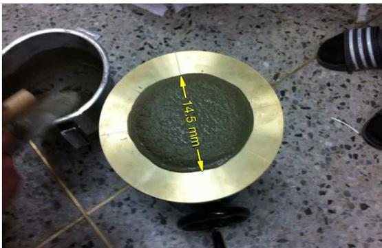
Figure 3 Liquidity test of the mortar with basalt powder sludge
