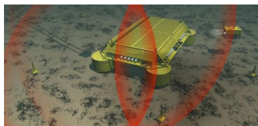
Fig. 1. Conventional Sonardyne® LBL system for work class ROV operation
