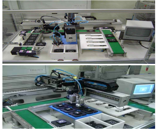
Fig. 5. Experimental scene for recognition of part shapes and character numbers
