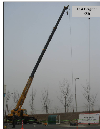
[Fig. 8] Site for Crash Impact Test [2]
