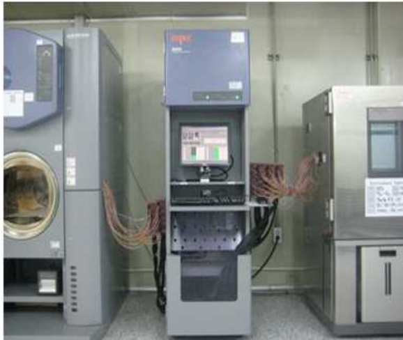
[Figure 3] Chamber, HAST Chamber and AMI
