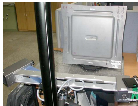
Fig. 2 Scanning of an automotive outer panel
