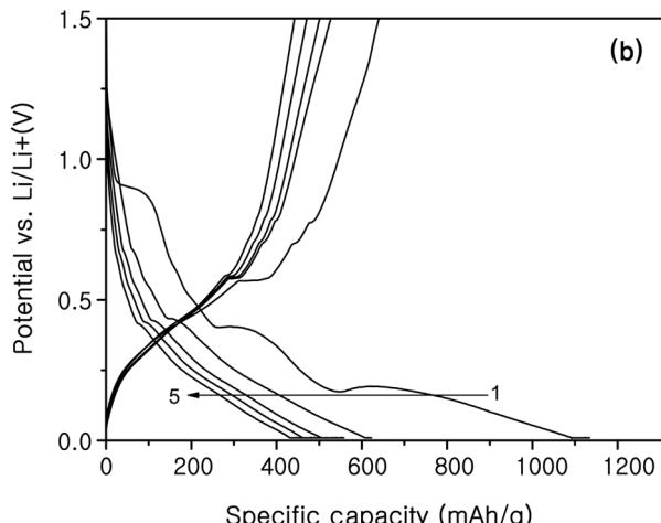
**Figure 7.** Charge-discharge curves of  $\text{SnO}_2\text{-SiO}_2$  composite with carbon coating at different heating conditions; (a)  $300\text{ }^\circ\text{C}$  and (b)  $900\text{ }^\circ\text{C}$ .
