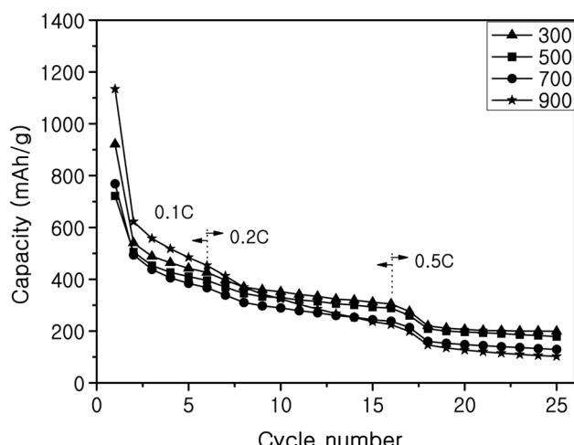
**Figure 9.** Cycle performance of  $\text{SnO}_2\text{-SiO}_2$  composite with carbon coating.
