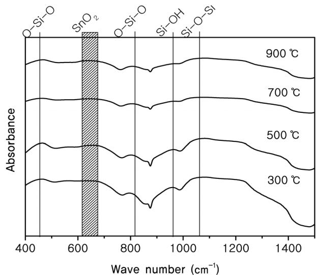
Figure 3. FT-IR spectra of SnO<sub>2</sub>-SiO<sub>2</sub> composite after heat treatment.
