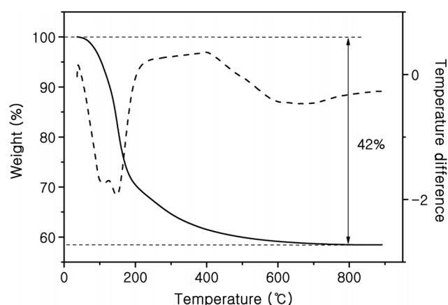
Figure 1. TG/DTA curves of SnO<sub>2</sub>-SiO<sub>2</sub> composite.
