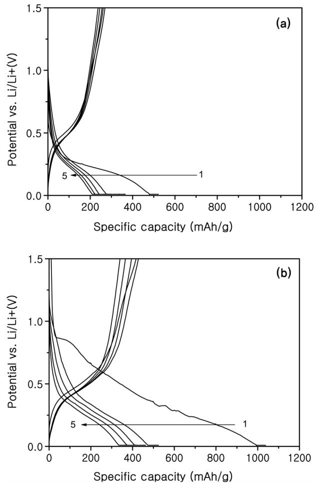
**Figure 6.** Charge-discharge curves of SnO<sub>2</sub>-SiO<sub>2</sub> composite without carbon coating at different heating conditions; (a) 300 °C and (b) 900 °C.
