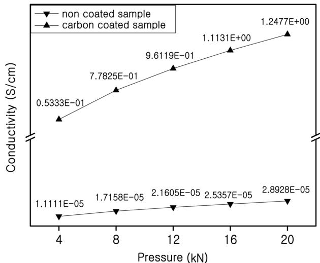
**Figure 5.** Electric conductivity of SnO<sub>2</sub>-SiO<sub>2</sub> heated at 300 °C.
