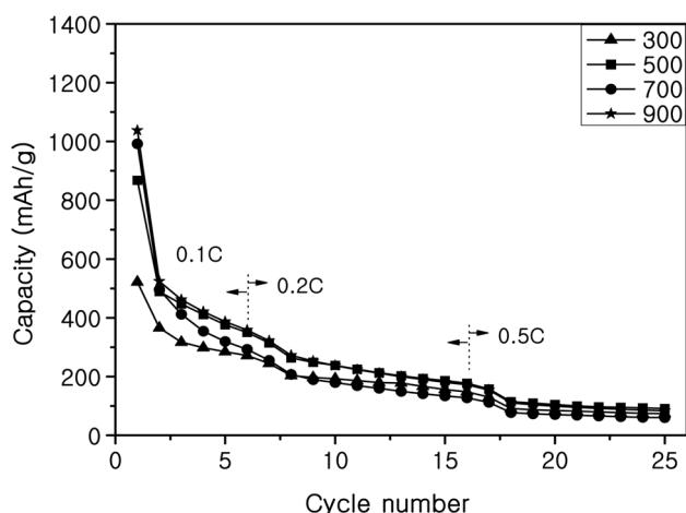
**Figure 8.** Cycle performance of  $\text{SnO}_2\text{-SiO}_2$  composite without carbon coating.
