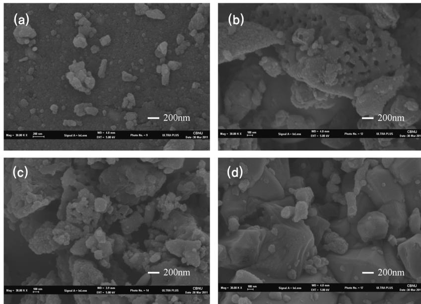
**Figure 4.** SEM images of SnO<sub>2</sub>-SiO<sub>2</sub>/C after heat treatment at (a) 300 °C( $\times$  30,000), (b) 500 °C( $\times$  30,000), (c) 700 °C( $\times$  30,000), and (d) 900 °C( $\times$  30,000).
