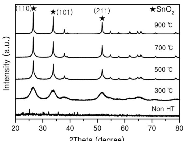
Figure 2. XRD patterns of SnO<sub>2</sub>-SiO<sub>2</sub> without carbon coating at different heat treatment temperature.
