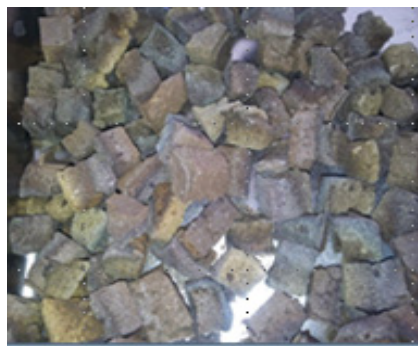
(e) quenching clinkers
