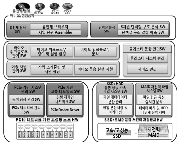
Fig. 11. Structure of MAHA system SW stack
