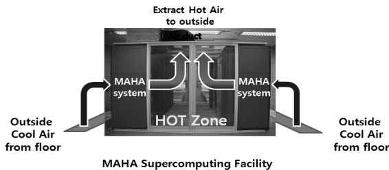
Fig. 17. HVAC implementation for MAHA supercomputing system
