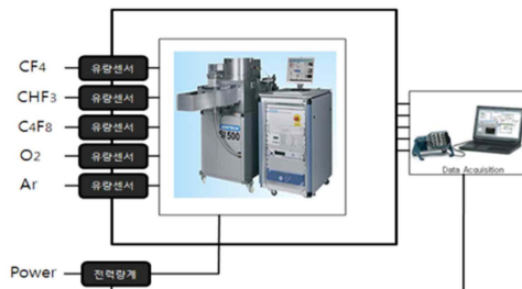
Fig. 1. Schematics of the experiment set-up for monitoring the energy and process gases consumption.
