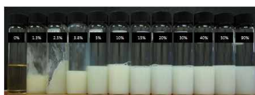
Fig. 1. Influence of increasing water concentration on the appearance, shear viscosity and electrical conductivity of emulsions at a fixed surfactant-to-oil ratio of 1.0.
