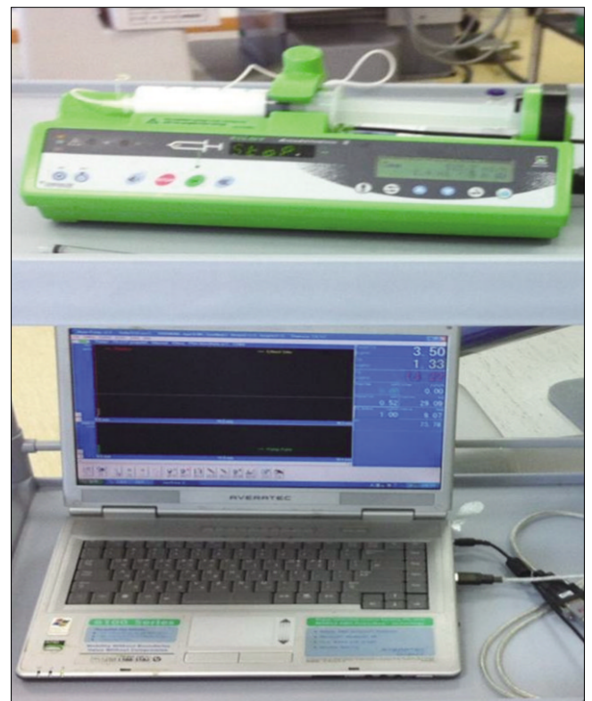
Fig. 2. Target controlled infusion device for propofol and a computer for the Asan pump program which is a microprocessor to run the pharmacokinetic modeling software and control the infusion device.
