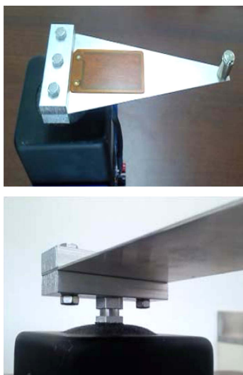
Fig. 5. Piezoelectric cantilever set up on top of electromagnetic shaker.
