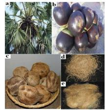
Fig. 1 (a) Borassus tree, (b) fruits, (c) dried fruits, (d) Borassus fruit coarse fibers and (e) fine fibers.
