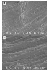
Fig. 2 SEM photographs of Untreated (a) and alkali treated (4 h) (b) Borassus fruit fine fibers.
