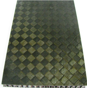
Fig. 4 Sandwich structure specimen.
