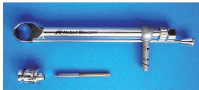
Figure 3. The appropriate driver was used to connect each spring-style mechanical torque device to the torque gauge.
