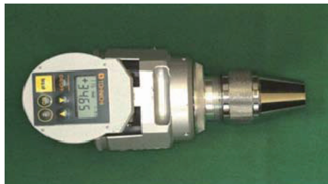
Figure 2. The digital torque gauge showing the peak torque at a predetermined target value designated by the manufacturers.
