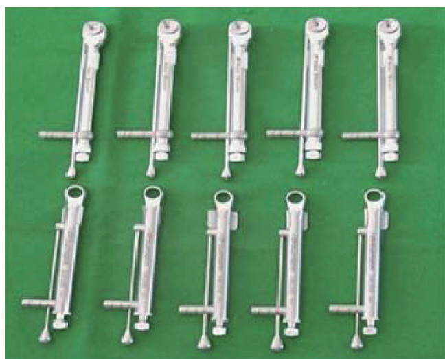
Figure 1. Spring-style mechanical torque devices tested in groups with dismantling and aging, and without. Top: Nobel Biocare, Bottom: Straumann (ITI).
