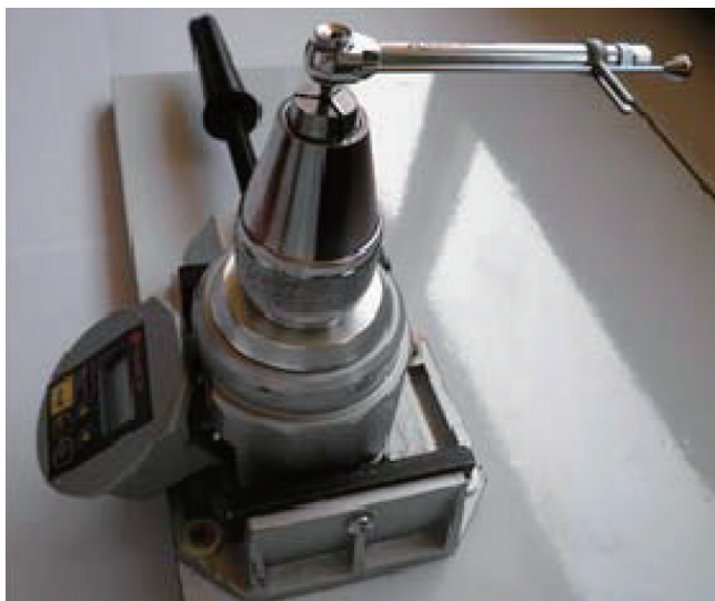
Figure 4. After connecting the devices to the appropriate drivers, they were clamped in a stable torque gauge.
