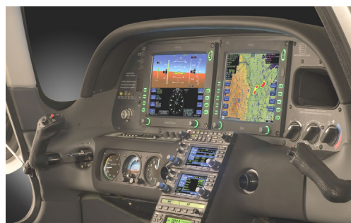
Fig 1. Glass Cockpit of Small Airplane
