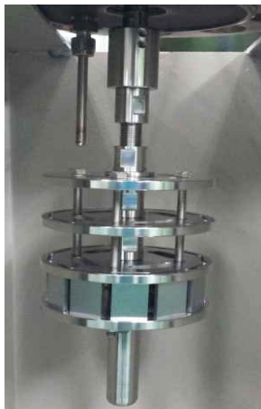
Fig. 2. FAC test specimen holder.
