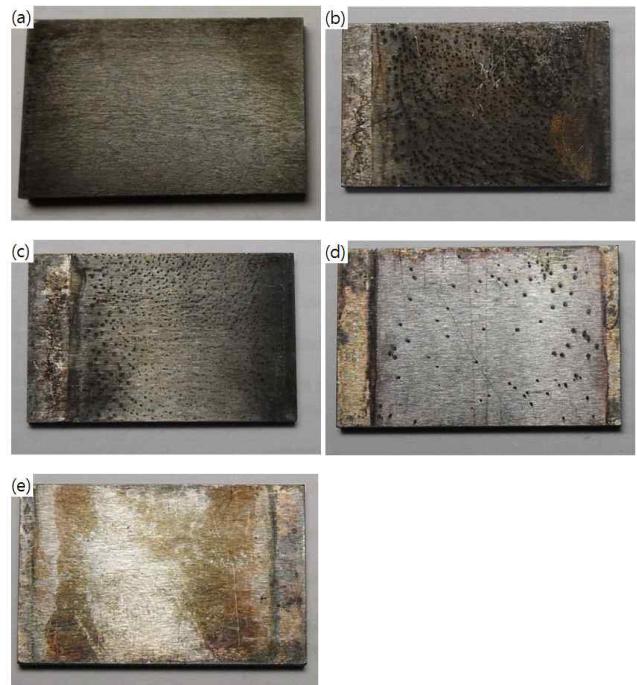
Fig. 3. Surface appearance after FAC test for 190 hours. (a) SA106 Gr.B; (b) SA508Gr.3; (c) A534 8620H; (d) SA508Gr.4N; (e) A336 F22V
