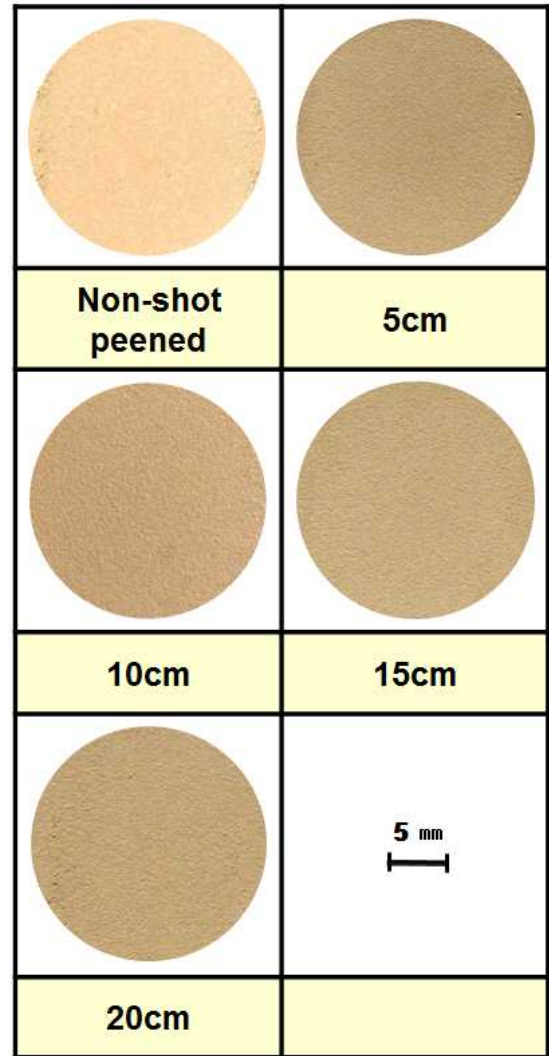
Fig. 3. Surface micrographs with stand-off distance after cavitation experiment in sea water for shot peened ALBC3 alloy.
