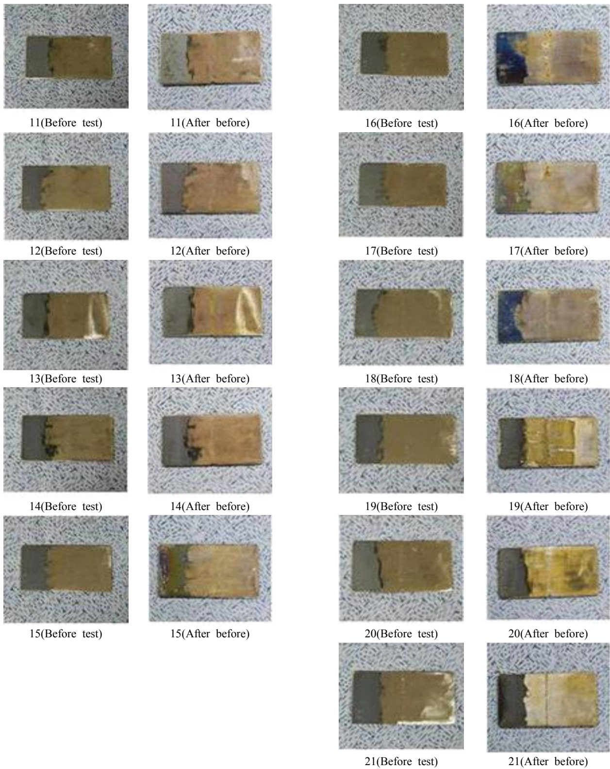
Fig. 4. The surface states of specimen after 720 hours corrosion tests.
