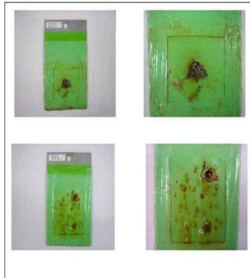
Fig. 11. The painted specimen by heavy paint coating systems.
