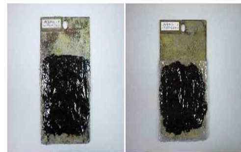
Fig. 8. Specimen of tar sealants coated.
