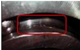
Fig. 4 Failure of ball bearing
