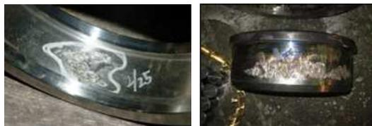
Fig. 2 Failure of roller bearing
