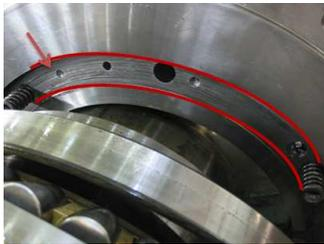
Fig. 1 Failure of thrust bearing
