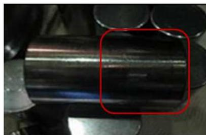
Fig. 3 Failure of roller bearing roller
