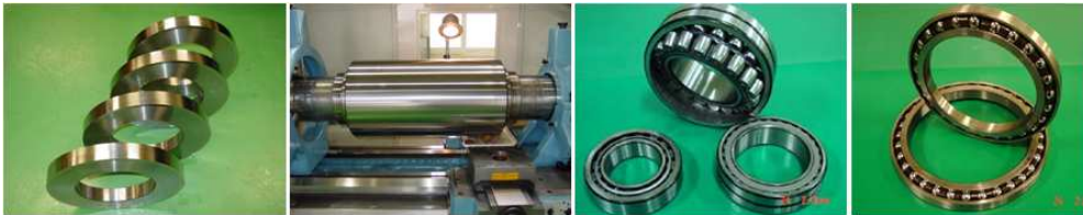
Fig. 7 Parts for the steel alloy which applied UNSM
