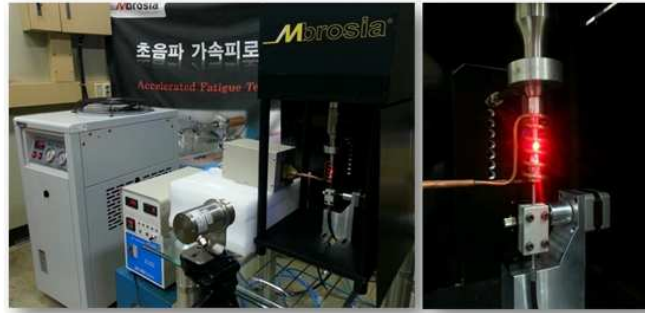
Fig. 10 System for ultrasonic fatigue test at high temperature
