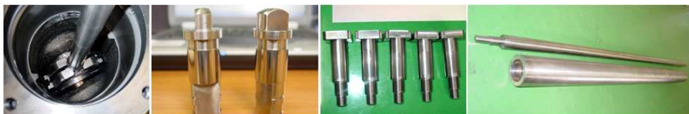
Fig. 8 High temperature structural material parts applying UNSM
