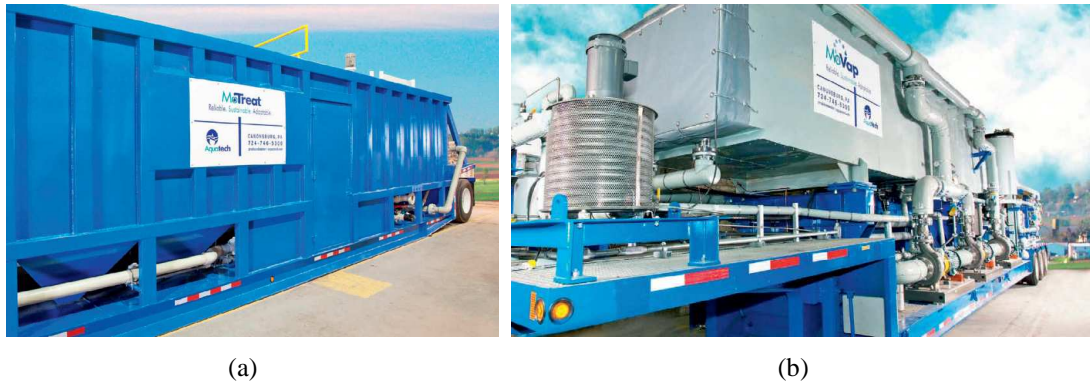
Fig. 2 Aquatech's mobile water treatment systems (30) : (a) pre-treatment, (b) thermal distillation
