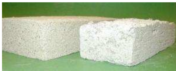
Fig. 4 Cementitious material for passive fire protection
