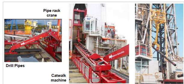
(b) Pipe handling system
