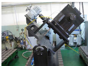
Fig. 13 Apparatus of the Heel 45° test rig condition
