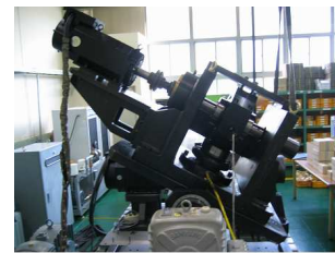
Fig. 15 Apparatus of Trim 30° test rig condition
