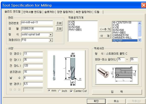
Fig. 12 An example of user interface for the cutting tool database
