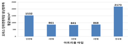
Fig. 7 Average cooling and heating load per unit volume of office by type
