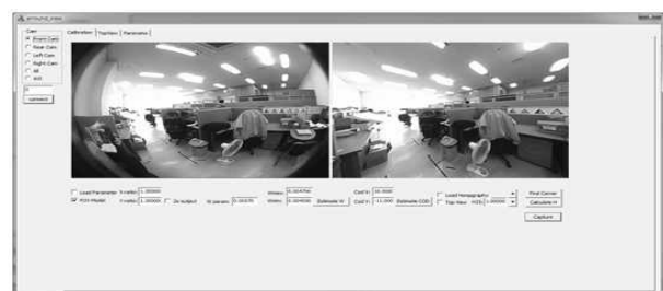
<Figure 6> Distorted image data of the camera by using the distortion correction parameters to a program
