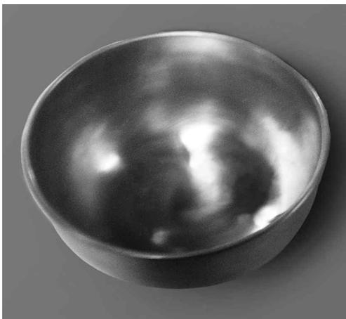
[Figure 12] Finish product with machining process using proposed safety shell mold
