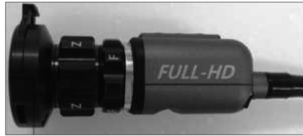
Fig. 1. A full HD CMOS camera was used to make a 2D scanning videokymography system.
