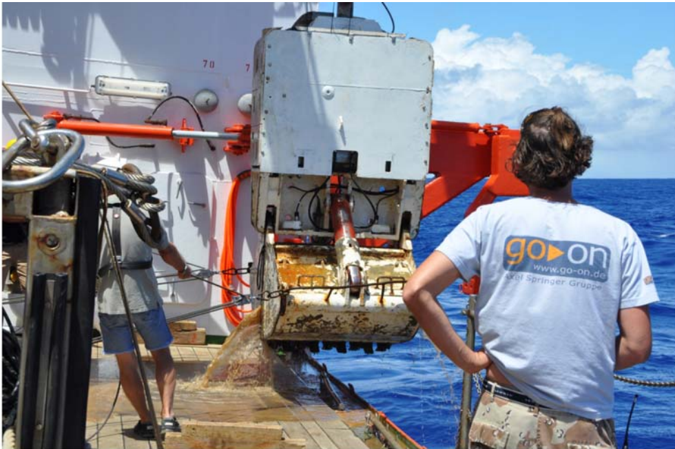
Fig. 2. Suspended surface sediments were flow out from TV guided grab sampler due to grab loosely.
