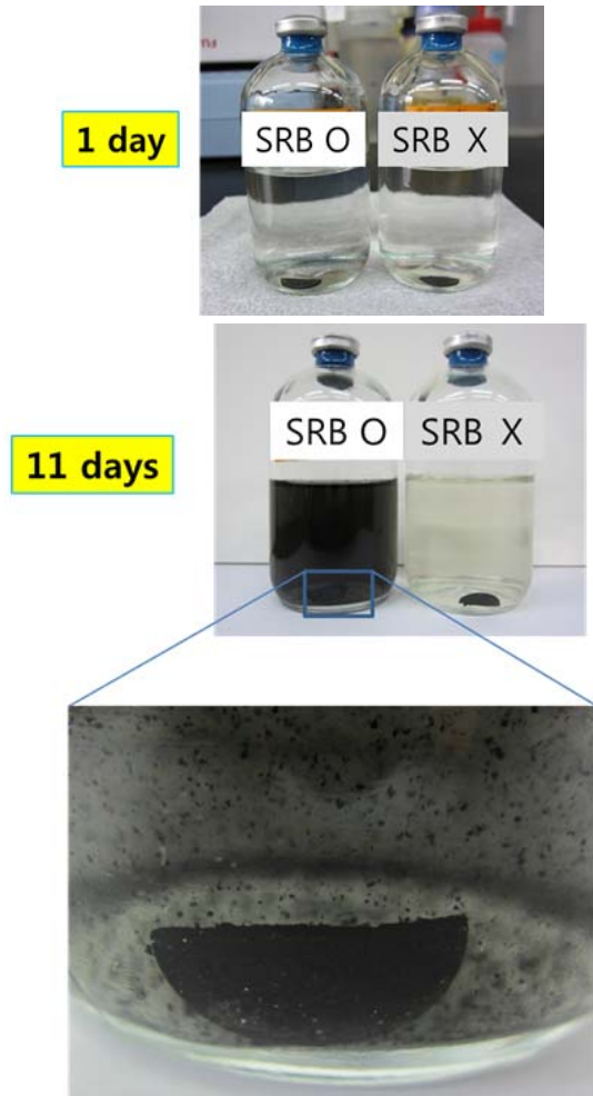
Fig. 1. A color change of serum bottles as a function of time, which contained a small cast iron plate specimen in a buffer solution with and without D. desulfuricans SRB.
