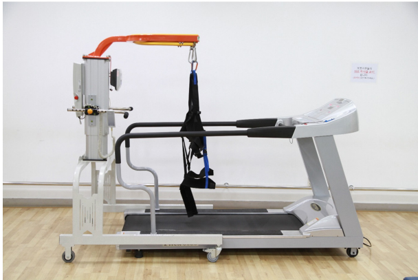
Figure 1. Device for body weight support (LINAK, Silkeborg, Denmark) and treadmill (FITEX T-5050; Fitex, Gwangju, Korea) and treadmill.
