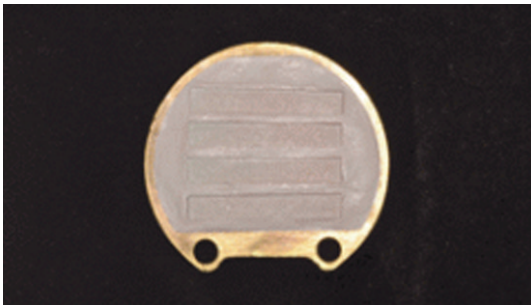
Fig. 2. Mold for fabricating resin specimens.
