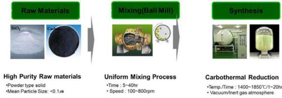
Fig. 5. Process map of the carbothermal reduction for ultra-high purity SiC powder.
