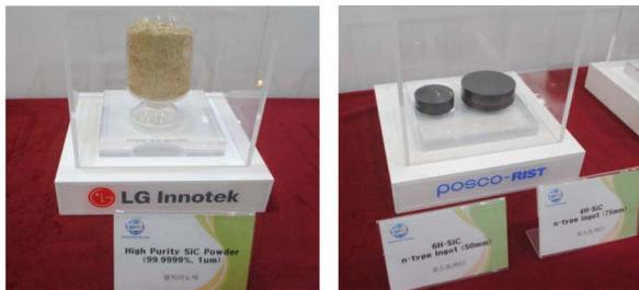
(a) Ultra-high purity SiC powder (b) 4H/6H SiC single crystal ingot
