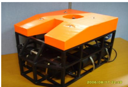
Fig. 1 Overview of hovering AUV
