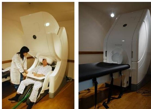
Fig. 1. Photographs of Vectorview (Elekta Neuromag Oy), helmet-shaped, 306-channel, whole-head neuromagnetometer installed in a magnetically shielded room at Seoul National University magnetoencephalography Center. The examination can be performed with the patient in a supine or a sitting position.
