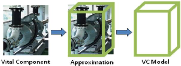
Fig. 5 Simplification of vital component by box model
