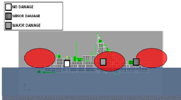
Fig. 3 Concept of damage ellipsoid analysis
