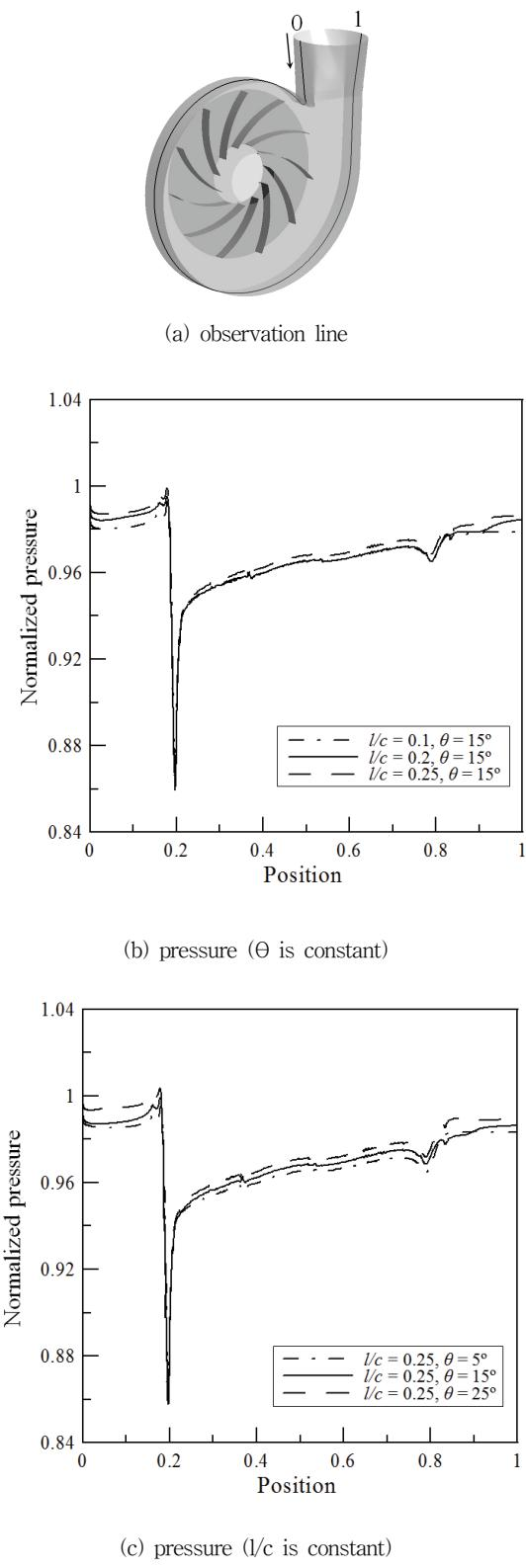
Fig. 9 Pressure along a volute casing
