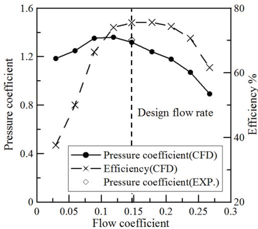
Fig. 4 Performance curve of a test blower<sup>(7)</sup>
