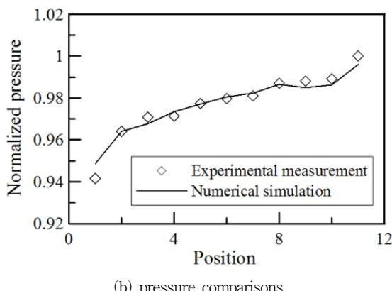
Fig. 5 Comparisons of pressure along the volute casing<sup>(7)</sup>
