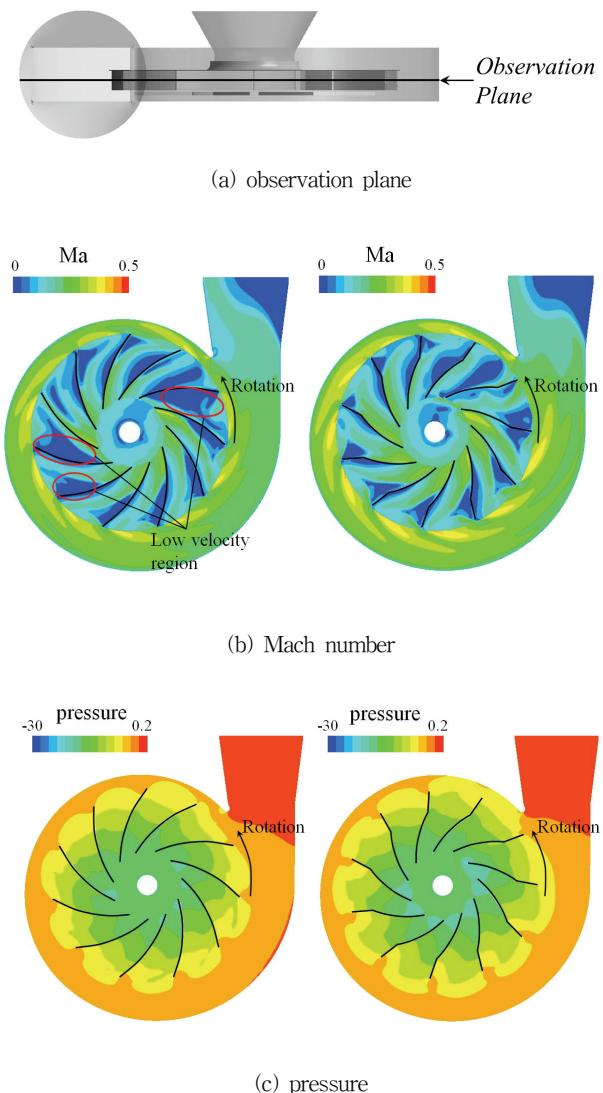
Fig. 10 Comparison of Mach number and pressure contours (left : reference blower, right : blower having max. pressure)
