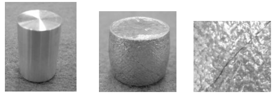
Fig. 1 Compression test of Al-Zn-Mg-Sc Alloy before heat treatment
