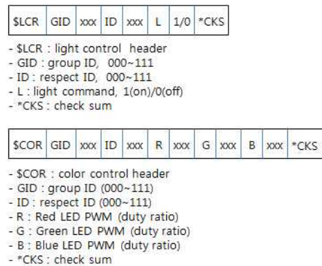
Fig. 6. Design of PWM frame.
