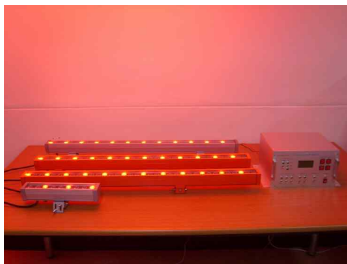
Fig. 9. Lighting test on red LED bar.
