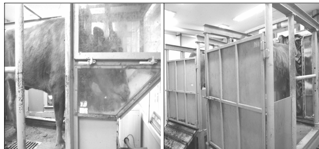
Fig. 1. Respiratory chamber of hood-type.
